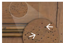
Wire Brush Holes Very small lightly patterned holes in different areas of a door
