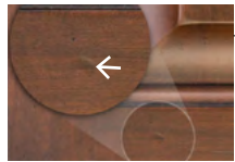
Dents Random placement of shallow dents
